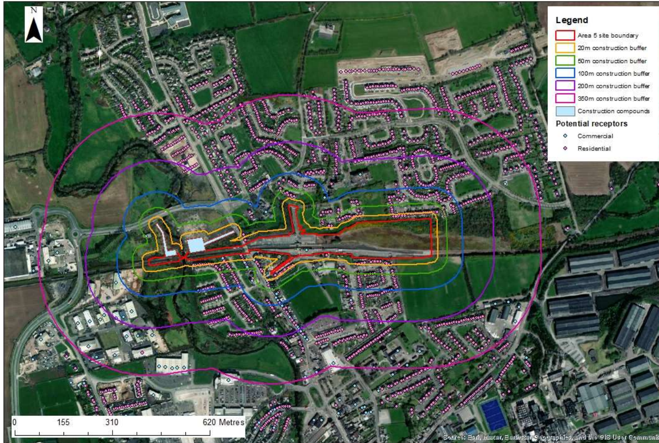
Figure 8.9: Construction Dust Assessment Buffers (Demolition, Earthworks and Construction) – Area 5
